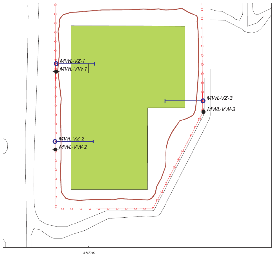
Figure 3.4.1-1 FLUTe™ Well Locations and Soil-Moisture Monitoring Access Tubes at the Mixed Waste Landfill
